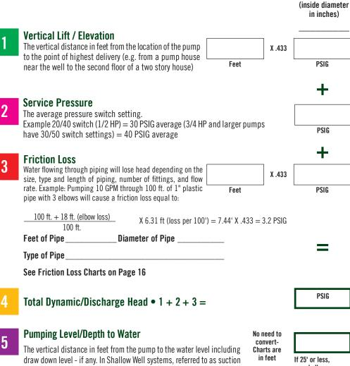
lift/head and is limited to 20 or 25 feet at sea level (deduct 1' suction capability for each 1000' above sea level).
