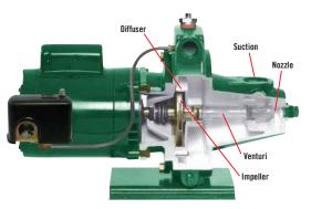
Centrifugal pumps, both the shallow-well and deep well types have little or no ability to pump air. When starting, the pump and suction line needs to have all of the air removed. An air leak in the suction line will cause the pump to quit pumping. This is sometimes referred to as "losing its prime".
