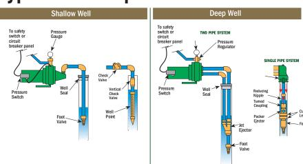
For a jet nozzle to be effective it must be combined with a venturi. The venturi changes the high-speed jet stream back to a high-pressure for delivery to the centrifugal pump. The jet and venturi are simple in appearance but they have to be well engineered and carefully matched to be efficient for various pumping conditions. The jet nozzle and venturi are also known as ejectors/ejector kits.
