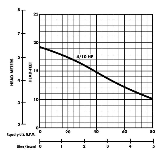
The curves reflect maximum performance characteristics without exceeding full load (Nameplate) horsepower. All pumps have a service factor of 1.2. Operation is recommended in the bounded area with operational point within the curve limit. Performance curves are based on actual tests with clear water at 70° F. and 1280 feet site elevation.
